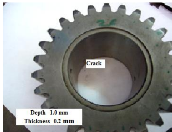
Fig.5 Wind turbine planetary gearbox healthy components Fig.6 Wind turbine planetary gearbox Planet gear tooth crake
